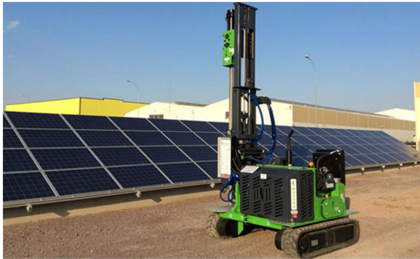
Figure 42: Machine to be Used for Fastening Panel Legs
